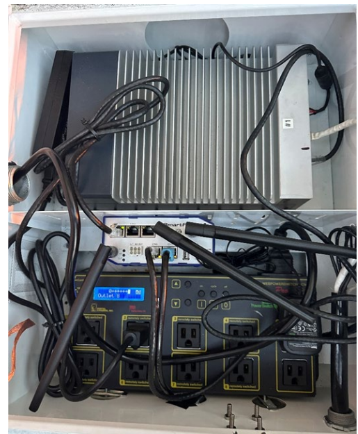
Cabinet assembly: AI Edge Processing and AI Mobile Edge Processing, includes a wireless 4G/5G router, AI edge processor unit, and web-managed power strip.
