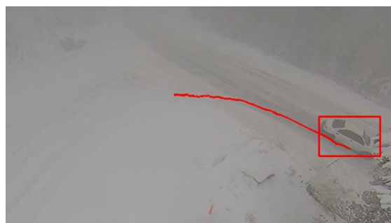
AI Sensor detecting wrong way driving in snow and low visibility conditions
